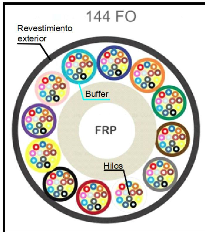
Figura 5. Cable ADSS Dielectrica Multitubo y Buffers
