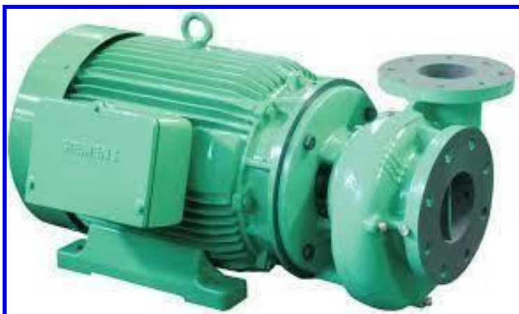
FIGURA N° 23: ELECTROBOMBA CENTRIFUGA ALTA PRESION 25.0 HP 3F 2.5"x2" 345 GPM@75m
