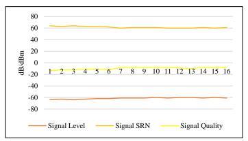
Figure 4: Antenna operational test 4GIC24371 20°
