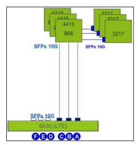
Figure 1: Equipment connection topology
