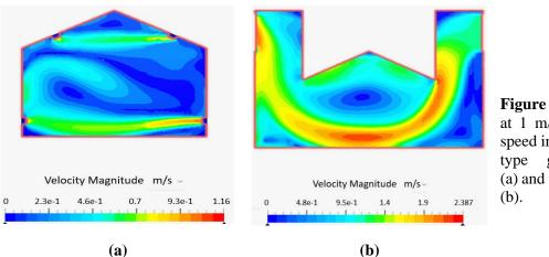
**Figure 4.** Air flow at 1 m/s entrance speed in triangular type greenhouse (a) and tunnel type (b).
