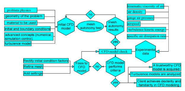
Figure 2. Procedure flow chart for simulation in SimScale CFD.
