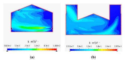
**Figure 7.** Turbulent flow with an inlet velocity of 1 m/s in triangular type greenhouse (a) and tunnel type (b).
