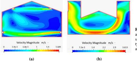
**Figure 5.** Air flow at 1.5 m/s entrance speed in triangular type greenhouse (a) and tunnel type (b).
