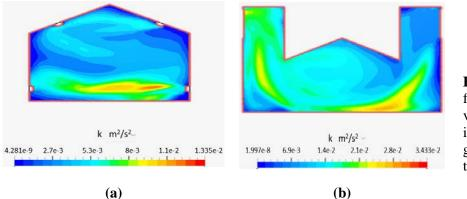
**Figure 6.** Turbulent flow with an inlet velocity of 0.5 m/s in triangular type greenhouse (a) and tunnel type (b).
