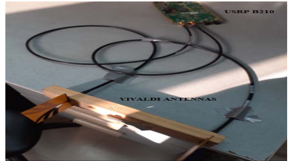
Fig. 4. USRP B210 and Vivaldi antennas for experiments
