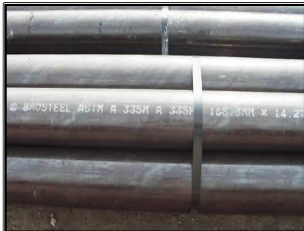
FIGURA N° 02: TUBERÍAS ALEADAS ASTM A335-P5
