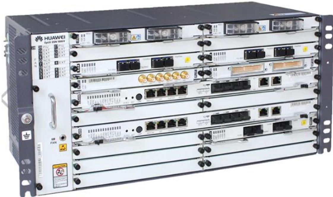
**Figura 28.** Huawei OSN 1800 V
