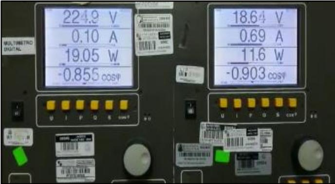
Figure 4: Electrical parameters per digital measurement module.
