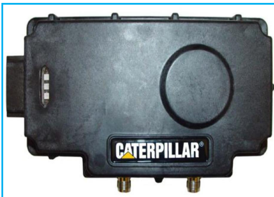
FIGURA N°11: RADIO SATELITAL PRODUCT LINK - GPS
