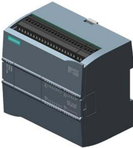
SIMATIC S7-1200, CPU 1214C, CPU COMPACTA, DC/DC/RELES, E/S INTEGRADAS: 14 DI 24VDC; 10 DO RELES 2A; 2 AI 0 - 10V DC, ALIMENTACION: DC 20,4 - 28,8 V DC, MEMORIA DE PROGRAMA/DATOS 75 KB
