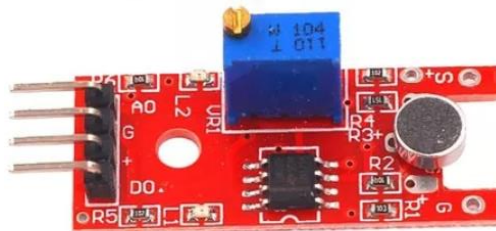
Figura 13: Módulo KY-038. Fuente: https://www.alldatasheet.com/datasheet-pdf/pdf/1138845/ETC2/KY-038.html
