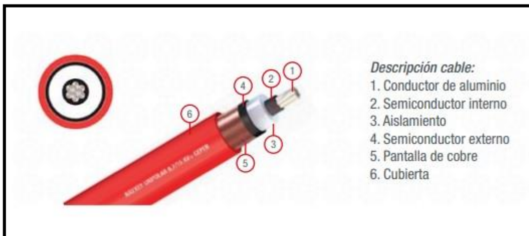
Figura N°8: Cable Unipolar NA2XSY.
