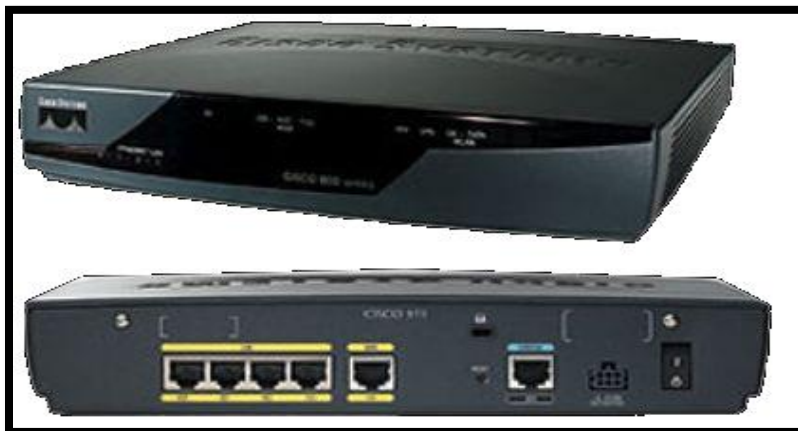
Figura 3.4: Router cisco 836 Fuente: https://goo.gl/rJvilZ
