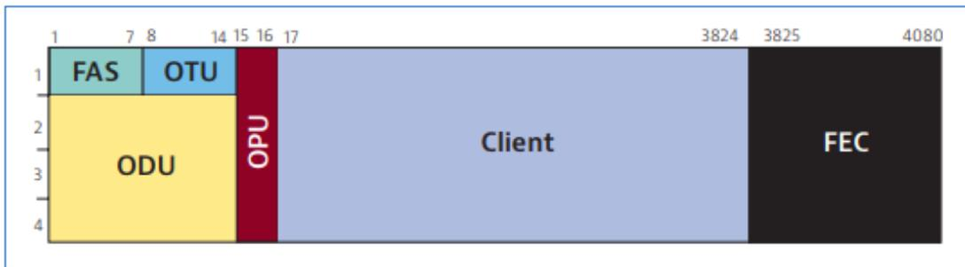
**Figura 2-32.** Estructura OTN (Schubert, A., s.f., G.709 – The Optical Transport Network (OTN). [FIGURE 6].Recuperado de <https://www.viavisolutions.com/ja-jp/literature/g709-optical-transport-network-otn-white-paper-en.pdf>)
