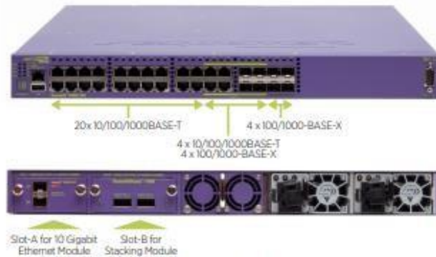
Figure 2: Summit X460-24t Flexible Port Configuration
