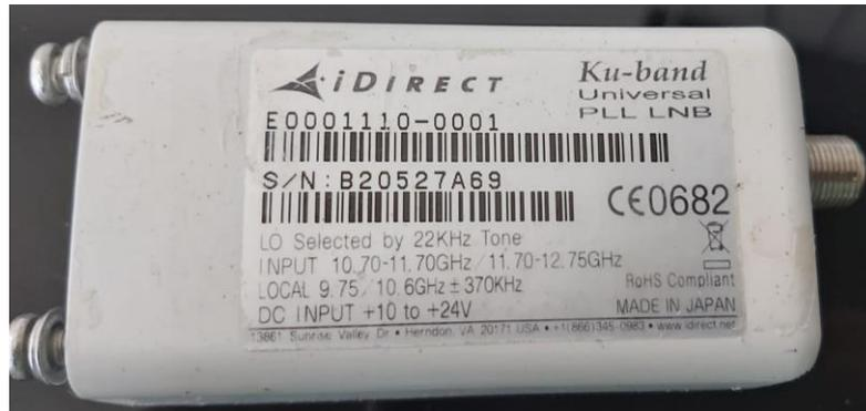
Figura 15: LNB iDirect, Banda Ku
