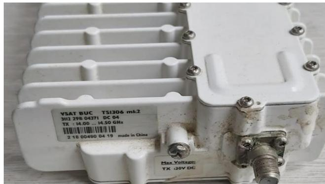
Figura 14: Block Up Converter 'BUC'
